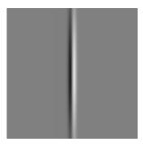
How can we combine oriented filters to signal an edge? The first-derivative operation takes the gradient of the image. From calculus, you learned that the gradient of a 2D function evaluated at (x,y) is a vector that points in the direction of maximum change. So taking the gradient of an image should produce a vector field where the vectors are perpendicular to the edges. The length of the gradient is a measure of the steepness of the intensity gradient.
