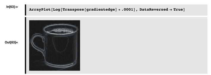
Doesn't look too bad, but it isn't clean and some of our satisfaction is premature and the result of our visual system effectively fitting the edge representation above into the interpretation of a cup. Further, we haven't specified a blur level, or a criterion for the threshold. We haven't put a measure of confidence on the edges.
